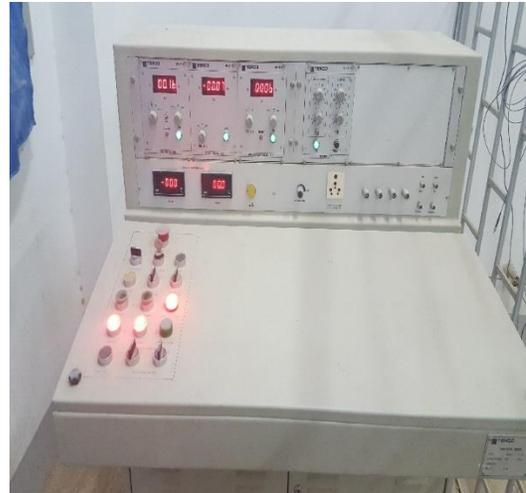
Figure 3: HV 9103 control desk includes measuring instruments and trigger device.
