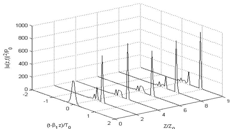
Figure 7: Decay of a second-order soliton ( $N = 2$ ) induced by intrapulse Raman scattering ( $\tau_R = 0.01$ )  $\tau_0 = 100fs$ ,  $z = 50\pi/2$ .
