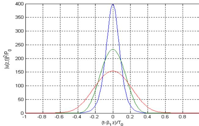
Figure 3: Dispersion-induced broadening of a Gaussian pulse inside Tellurite Glass Codoped  $\text{Er}^{3+}/\text{Tm}^{3+}$  with  $\beta_2 = 7.92e - 5 \text{ ps}^2/\text{m}$ ,  $\tau_0 = 100\text{fs}$ ,  $L_D \approx 162\text{m}$
