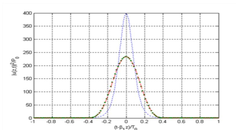
Figure 5: Pulse shapes at  $z = 200L'_D$  of an initially Gaussian pulse at  $z = 0$  (solid curve) in the presence of  $\beta_2$  second order dispersion. Dashed curve shows the effect higher order dispersion  $\beta_2$  and  $\beta_3 \neq 0, \tau_0 = 100fs$
