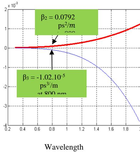
Figure 2: Variation of  $\beta_2$  and  $\beta_3$  with wavelength for Tellurite glass Codoped  $Er^{3+}/ Tm^{3+}$ .
