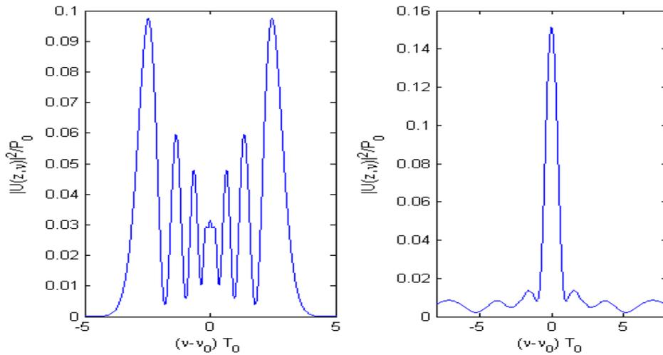
Figure 4: SPM-broadened spectra for an unchirped Gaussian pulse. Spectra are labeled by the maximum nonlinear phase shift  $\Phi_{max}$ . (in the left for Gaussian pulse  $m=0$ , and right for super-Gaussian pulse  $m=3$ ),  $\tau_0 = 100fs$ ,  $L_{NL} = 7.14 m$
