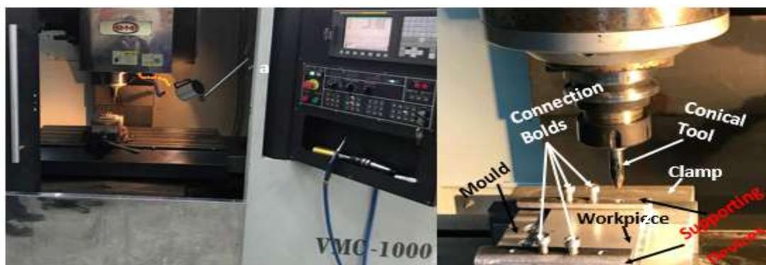
Figure 1: a) CNC milling machine and its computer screen, b) experimental setup
