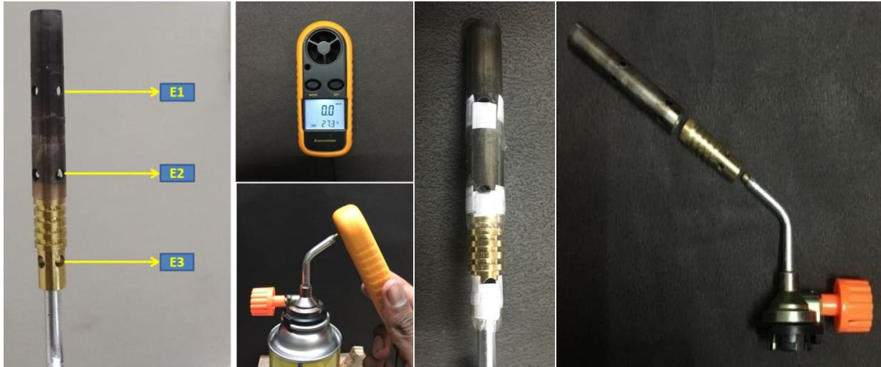
Figure 3: Essential components of experimental setup (left to right) viz., nomenclature of array of holes, Anemometer and flow measurement, All open case, Removable sub-parts of nozzle
