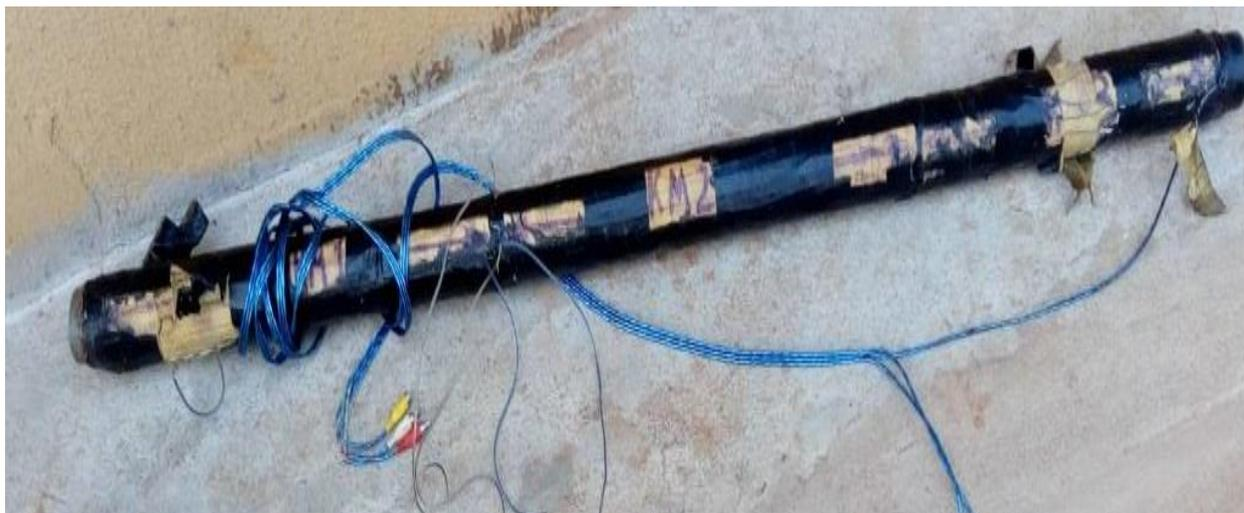
Figure 1: Sample petroleum pipeline coated with sensor wires
