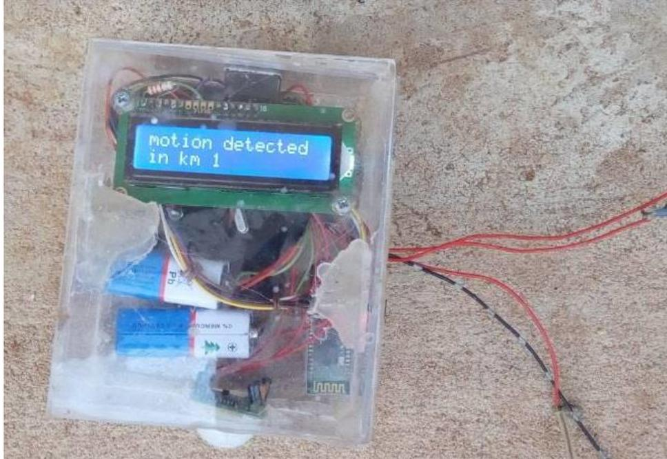
Figure 7: Complete designed prototype packaged in a case
