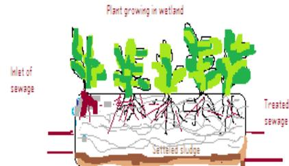
Fig.1 Constructed Wetland flow chart
