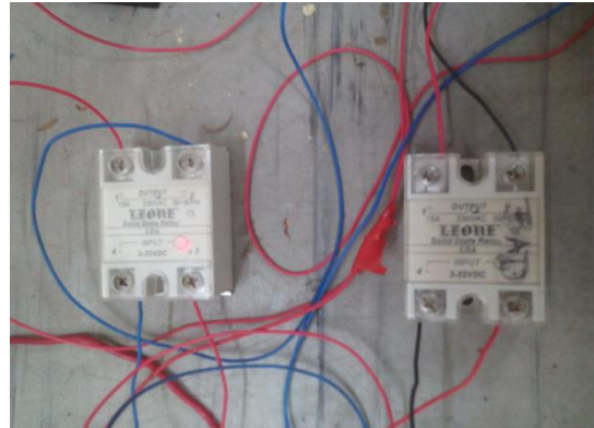
Figure 6: When SSR1 is ON and SSR2 is OFF.
