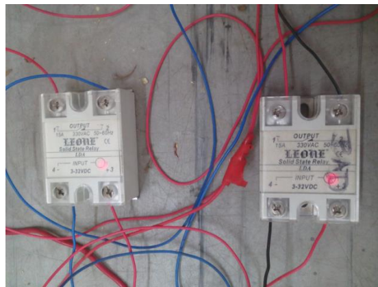
Figure 8: When SSR1 and SSR2 are ON.
